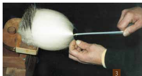
1a and 1b) Plank the top by breaking it into 30" lengths to be regrouped, lashed onto the comb, and combed one more time. Planking redistributes fiber lengths to make the final top more consistent. 2) Use a diz with a large hole for coarse wool, such as Border Leicester. 3) Use a diz with a small hole for fine wools such as Polwarth.
