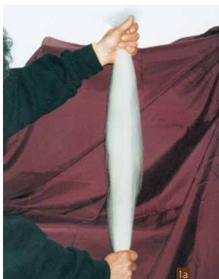
1a and 1b) Plank the top by breaking it into 30" lengths to be regrouped, lashed onto the comb, and combed one more time. Planking redistributes fiber lengths to make the final top more consistent. 2) Use a diz with a large hole for coarse wool, such as Border Leicester. 3) Use a diz with a small hole for fine wools such as Polwarth.
