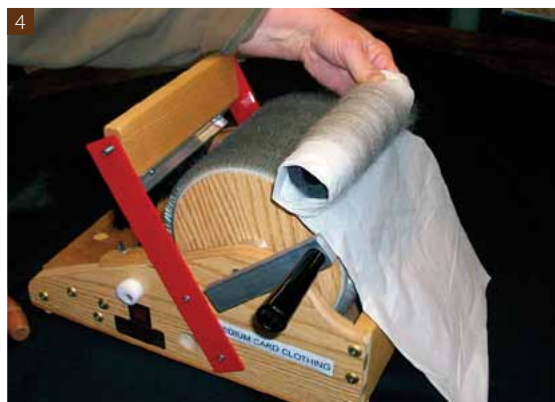
1) Locks and teased fiber. 2) Teased locks being fed into carder. 3) Use the doffer to gently break the batt apart at the seam in the card clothing. 4) Roll the batt off the drum using a paper towel tube. PHOTOS BY ROBIN RUSSO
