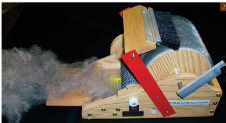
1) Locks and teased fiber. 2) Teased locks being fed into carder. 3) Use the doffer to gently break the batt apart at the seam in the card clothing. 4) Roll the batt off the drum using a paper towel tube. PHOTOS BY ROBIN RUSSO
